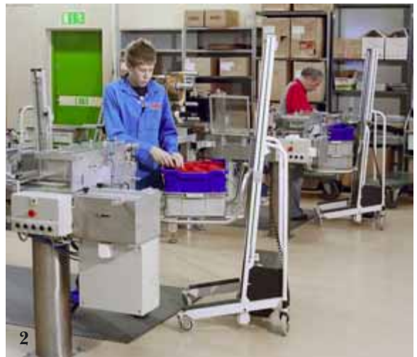
2. These PRO100's are used as mobile work stations in this assembly line.
