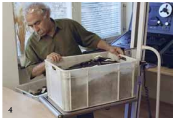
4. A roller on the front of the platform simplifies the loading and unloading of this PRO70.
