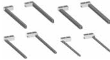
8152A/B/C/D Adjustable forks for PRO120/150 frame 8102A. A: 80 kg 40x20 mm l: 500 mm. B: 60 kg 30x30 mm l: 500 mm. C: 40 kg 20x20 mm l: 400 mm D: 40 kg dia 25 mm l: 450 mm. Reaches floor level.
