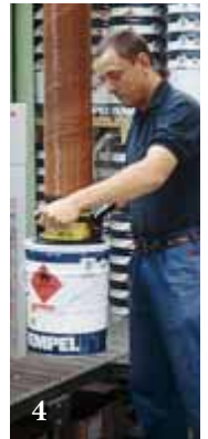
4. A VacuEasylift that lifts drums/tins/buckets is a popular installation in the pharmaceutical/chemical industries. We deliver suction feet for handling one or more tins at a time.
