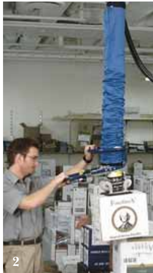
2. Retailers of alcoholic beverages use the VacuEasylift to handle boxes, crates and kegs. These units are equipped with a specially designed handle and are delivered with lightweight, lowbuilt aluminium jib cranes and crane systems.
