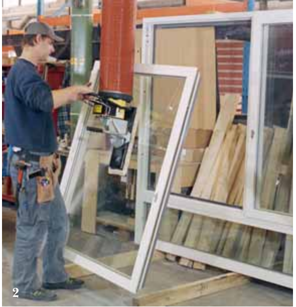
1-2. The suction feet used to lift panels and boards vary in design due to variations in size, weight and density of material. In some cases two suction feet on a wide yoke is sufficient. This also applies to all types of window handling.
