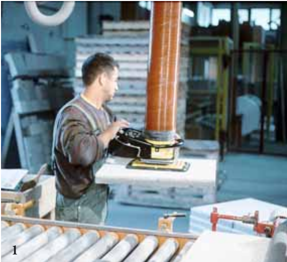
1. VacuEasylift relieves strained shoulders and backs in the heart of building and landscaping materials industry.
