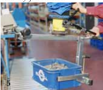
5. A VacuEasylift with a special tool attached for handling crates. This particular unit is equipped with a fast coupling to allow fast changes between the crate tool and another suction foot for boxes.
